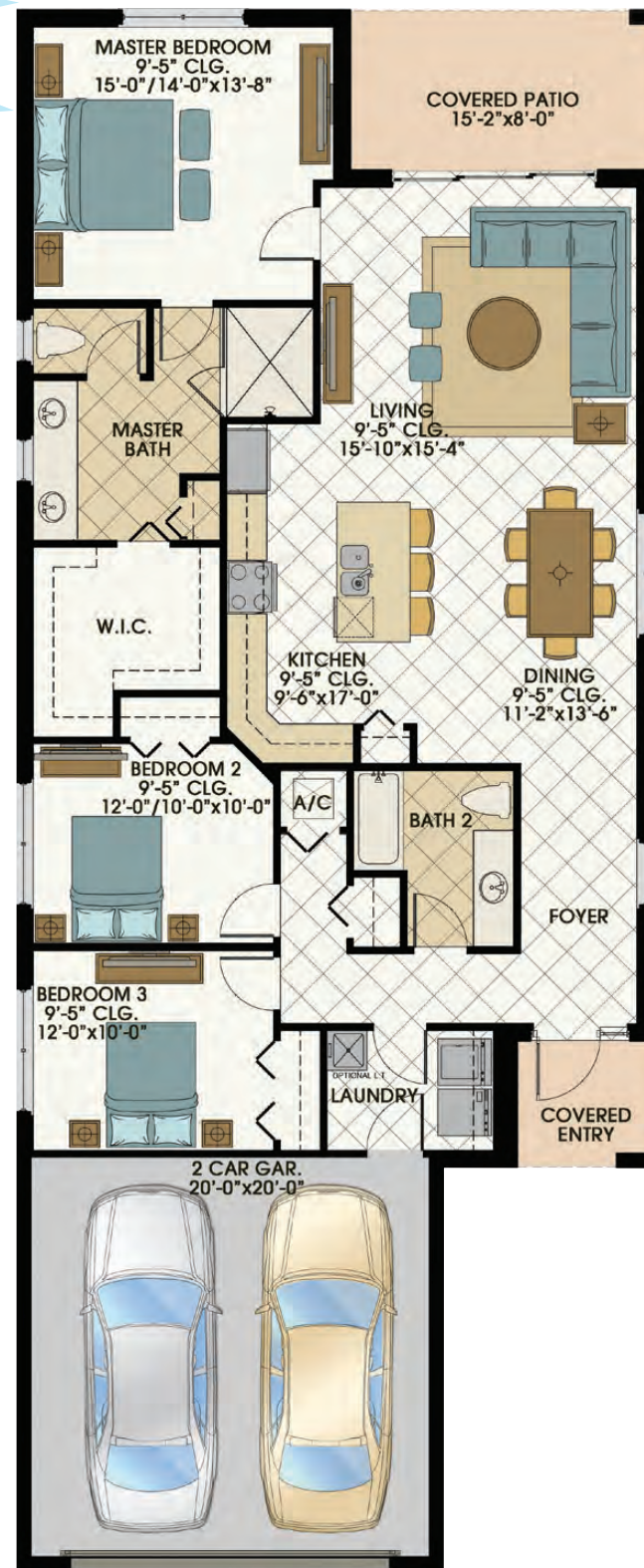
1ST FLOOR PLAN
